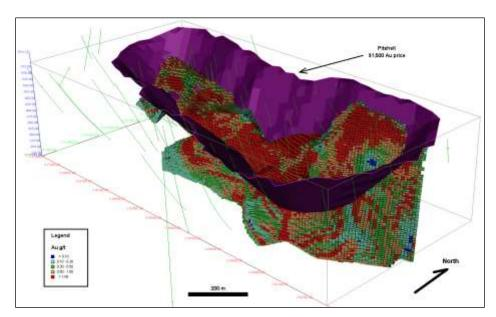
Figure 14.10 Candelones Extension Block Model Isometric View
