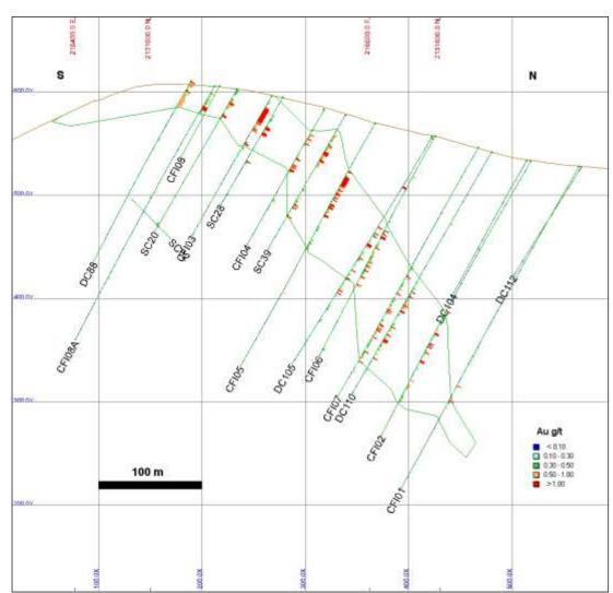
Figure 10.5 Cross-Section of Significant Drill Holes CF103, CF104, CF105 and CF107 on the Candelones Main Zone
