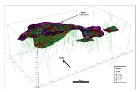
Figure 14.9 Candelones Main and Connector Block Model Isometric View
