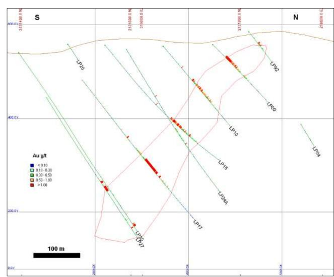
Figure 10.4 Cross-Section of Significant Drill Holes LP09, LP10, LP15 and LP17 on the Candelones Extension Zone
