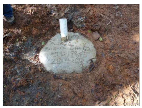
Figure 10.2 Concrete Monument for a Drill Hole
