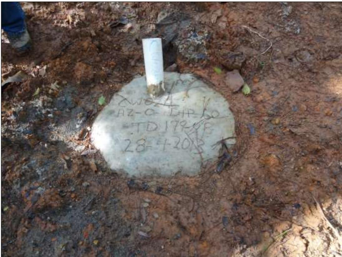
The monuments are surveyed using differential GPS survey instruments at a later date and the more accurate survey data are supplied to the database manager, who updates the final collar location in the database.
