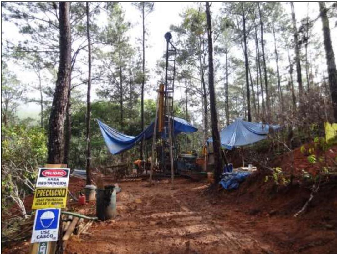
Drill locations are selected by the Qualified Person managing the Project. Platform locations are located in the field, utilizing hand held GPS receivers. After the platforms are constructed, the collar location for the drill hole is established and the drill is moved onto the platform and aligned by a Qualified Person.
