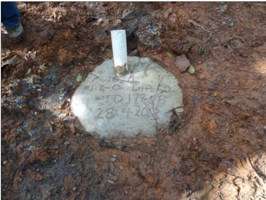
Figure 10.2 Concrete Monument for a Drill Hole
