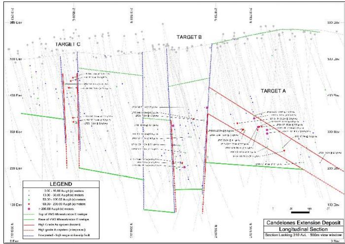
Figure 10.4 Simplified Longitudinal Section A – A' CE Deposit
