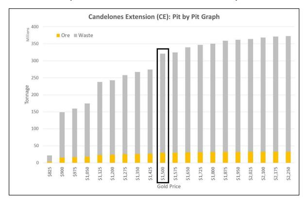
Figure 1.4 Simple Revenue Factors for each Nested Pit Shell for the CE Deposit
