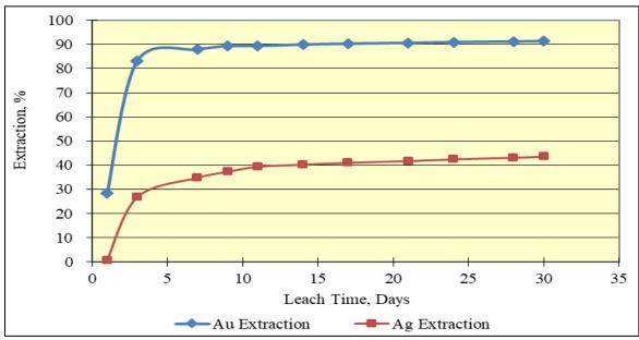
Figure 13.2 Oxide Composite – Column Cyanide Leach Test Results
