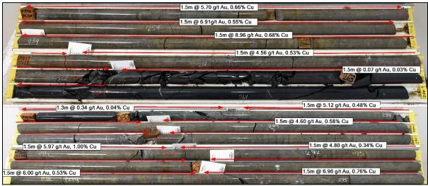
Figure 7.9 Massive Sulphide with Mafic Dike – LP19-132M Target A – CE
