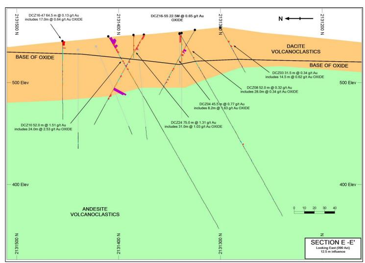
Figure 10.8 Simplified Cross-Section E-E' CMC Deposit
