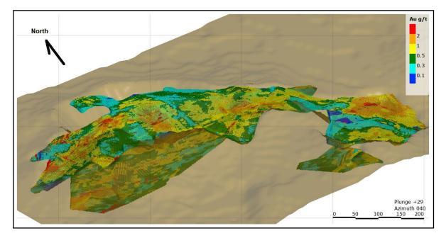
Figure 14.9 CMC Block Model and US\$1,500 Pitshell Isometric View
