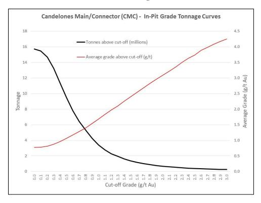
Figure 14.16 CE Grade/Tonnage Curve
