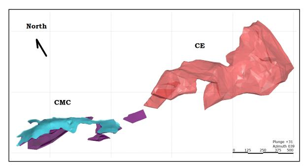
Figure 14.2 Finalized Wireframes for the Three Candelones Mineral Zones
