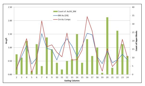
Figure 14.14 Results for the CE Zone Swath Plot, Composite versus Block Model
