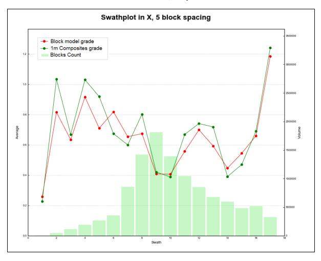
Figure 14.13 Results for the CMC Zone Swath Plot, Composite versus Block Model
