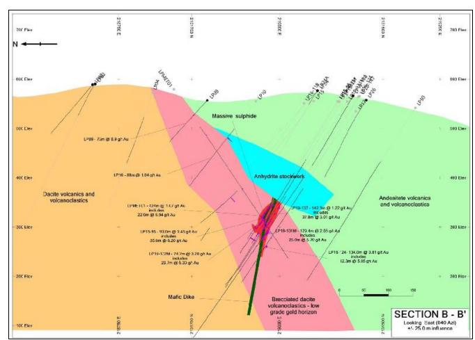
Figure 10.5 Simplified Cross-Section B-B' CE Deposit, Target A
