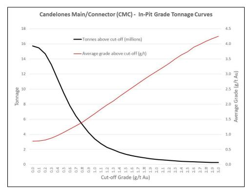
Figure 1.1 CMC Grade/Tonnage Curve
