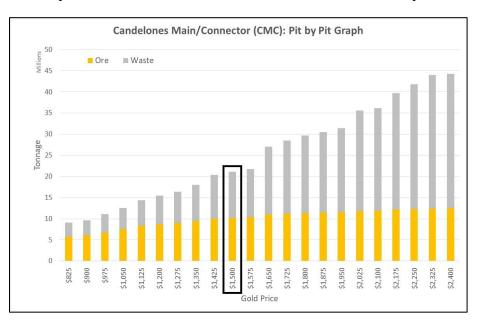
Figure 25.3 Simple Revenue Factors for each Nested Pit Shell for the CMC Deposit
