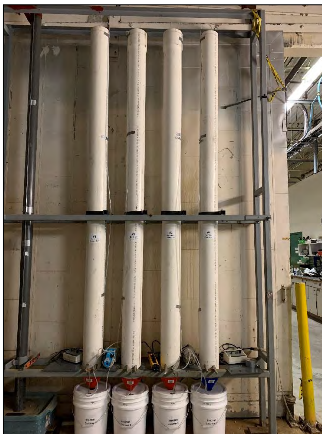
Figure 13.4 Photograph of the BVM Column Leach Test Setup
