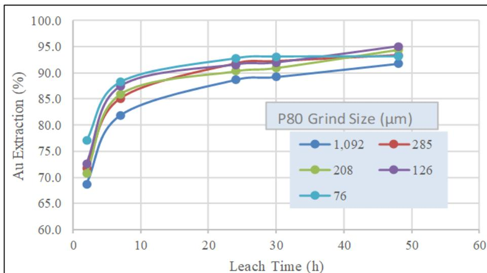
The bottle roll leach tests show that the oxide mineralization is amenable to standard agitation cyanide leach technology, even at relatively coarse grind sizes. These results suggest that there is limited benefit with regard to gold leach recovery with grinding finer than 285 microns.
