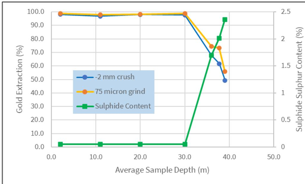
The gold dissolution for the variability samples followed a similar trend as that for the main composites. The finer ground samples did achieve faster kinetics and slightly higher overall dissolutions, on average. Reagent consumptions were similar to the zone composites.
