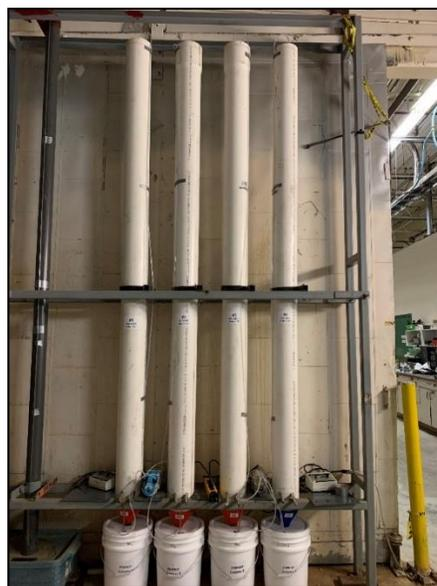
The two oxide columns were leached for 44 days, whilst the transition and sulphide columns were leached for a total of 79 days. The gold extraction results for all four column tests are presented in Figure 13.16 and Figure 13.17. The column test results are based on final residue sample analyses.
