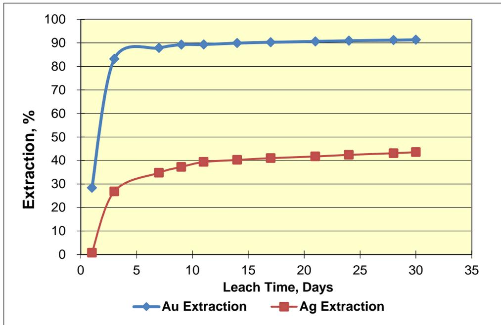
It can be seen from Figure 13.11 that effective leaching was completed within 20 days and that excellent gold dissolution of the order of 90% would be expected to be achieved. In addition reasonable silver dissolution of the order of 40% could be expected. The cyanide consumption kinetics are presented in Figure 13.12.
