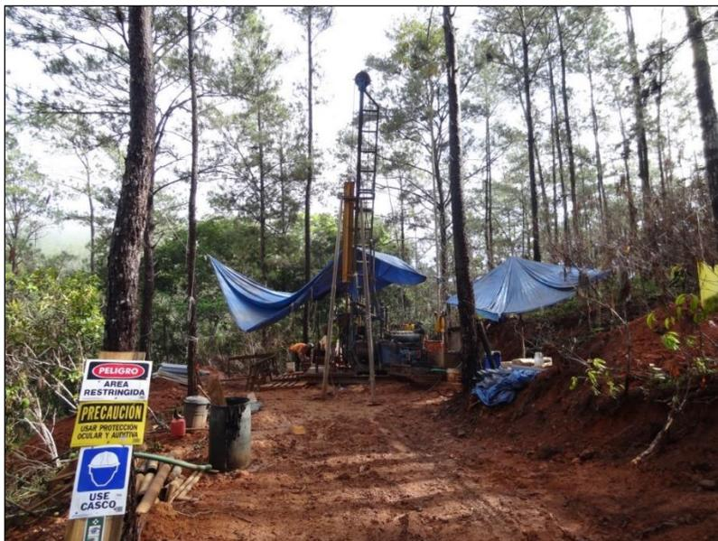
Drill locations are selected by the QP managing the Project. Platform locations are located in the field, utilizing hand-held GPS receivers. After the platforms are constructed, the collar location for the drill hole is established and the drill is moved onto the platform and aligned by a QP.
