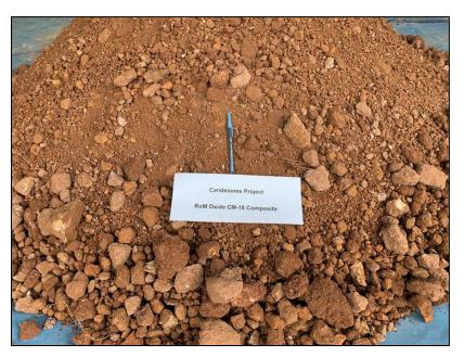
Figure 13.9 ROM Composite CM-18 Sample for Column Testing
