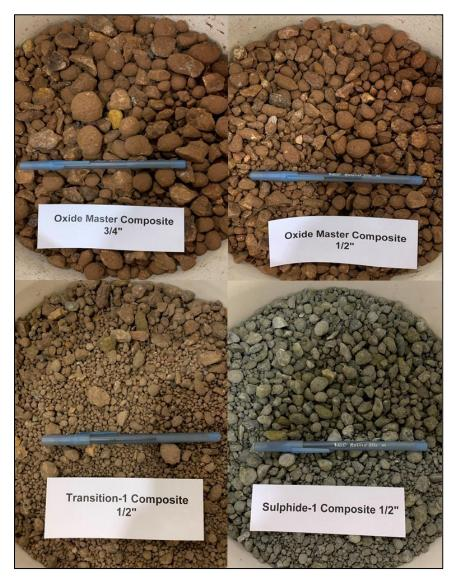
Figure 13.8 Phase 2 Column Feed Material after Agglomeration
