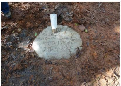
Figure 10.2 Concrete Monument for a Drill Hole
