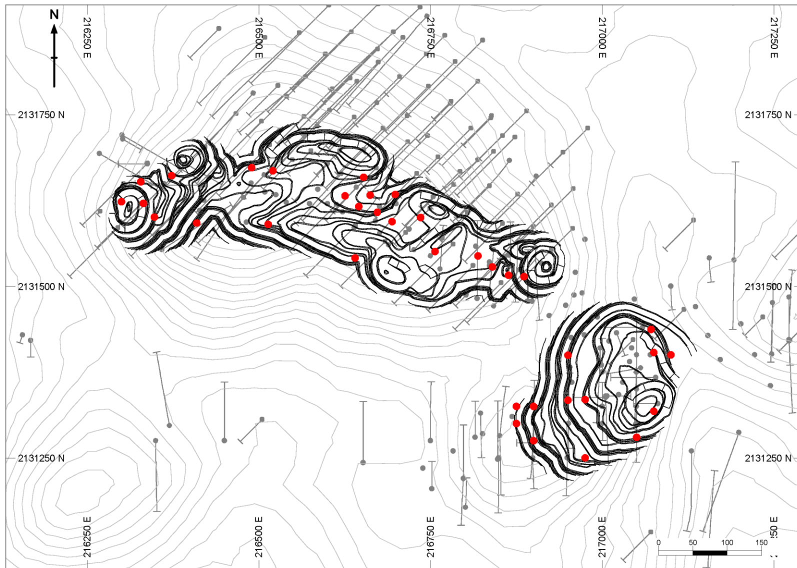
Figure 1.0 - Candelones Oxide Pit Area showing historic drilling and collars of recent infill drilling
