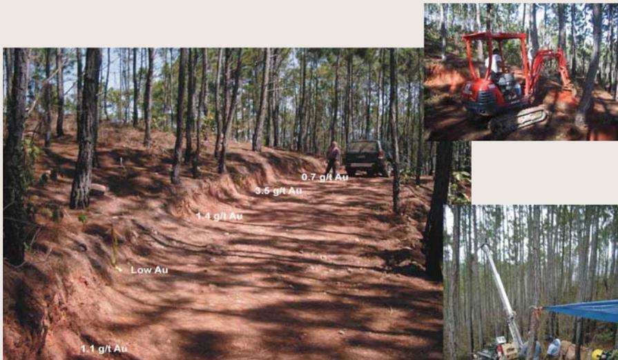
58 diamond drill holes into a 1200 m by 600 m coincident gold-in-soil anomaly and IP chargeability high. Trenching to 26.3 g/t Au over 16 metres and diamond drilling to 4.4 g/t Au over 25 metres. Chip sampling along drill access road in E-W direction ran >1 g/t gold over 200 metres.
